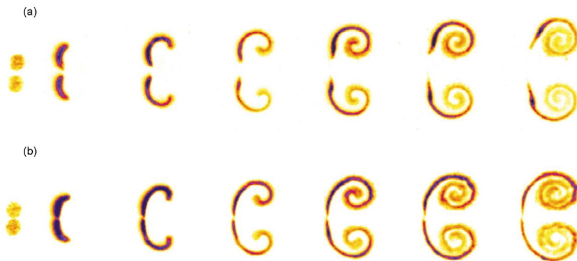
Fig. 8. Examples of double-cylinder flow morphologies: strong interaction. Images are acquired at t = 0 , 50, 190, 330, 470, 610 and 750 m s after shock impact. Legend as in Fig. 4. (a) S = 1.4D ; (b) S = 1.2D .
