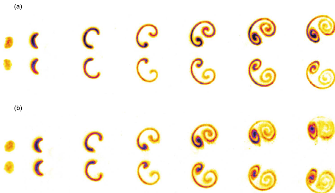
Fig. 6. Examples of double-cylinder flow morphologies: weak interaction. Images are acquired at t = 0, 50, 190, 330, 470, 610 and 750 \text{ ns} after shock impact. Legend as in Fig. 4. (a) S = 2.0D ; (b) S = 1.8D .
